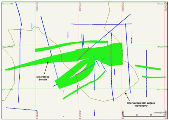
Figure 14-10: Central Breccia Plan Section 470, showing vein strike orientation and intersection with surface topography
