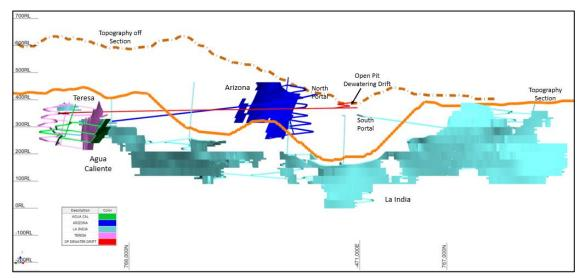
Figure 16-24: La India UG Design Long Section View (Modified North and South Portals)
