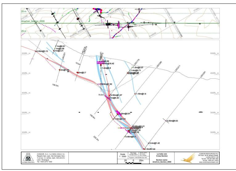
Figure 7-9: Cross-section through the intersection of the Constancia Vein with the America-Escondido flexure with the Constancia Vein(s) on the 500 Section (Source: Condor 2014)
