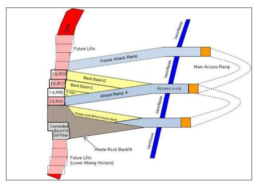
Figure 16-20: Mechanized Cut and Fill Section View (SRK, 2021)
