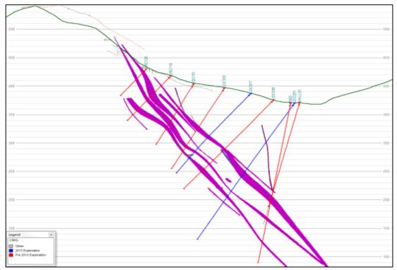
Figure 10-5: Cross section (Section Line - 850) through the La India-California veins showing holes drilled to the SW, confirming the width of ore zones (Source: SRK)
