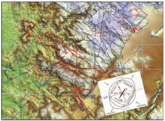
Figure 7-4: Interpretation of brittle structures and lineaments in the core mineralised area at La India over topography image.
