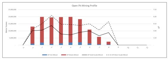
Figure 1-1: Scenario 1 Open Pit Only Mine Plan
