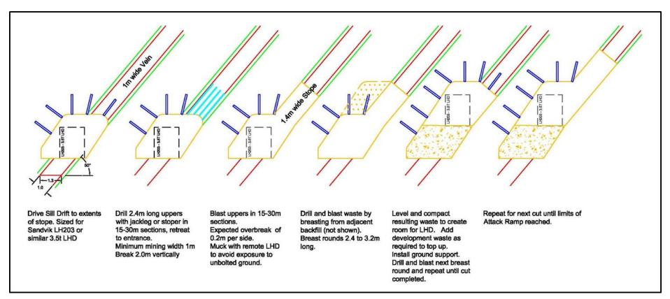
Figure 16-21: Illustration of MCF Mining Method with Resuing (SRK, 2017)
