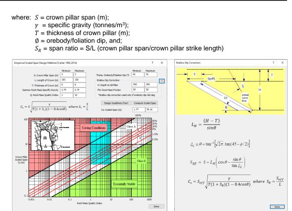
Figure 16-2: Empirical Scales Span Design Method (Carter 1992, 2014)
