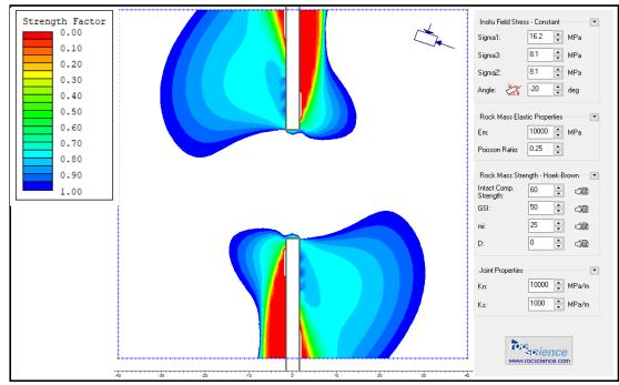
Figure 16-4: Example Strength Factor plot of 2D elastic analysis of sill pillar
