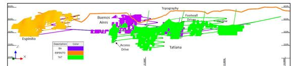
Figure 16-28: Mestiza UG Design Long Section View
