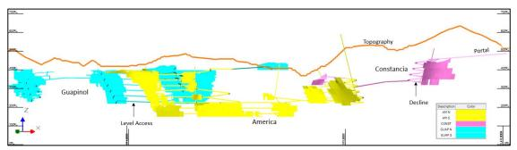
Figure 16-26: America UG Design Long Section View
