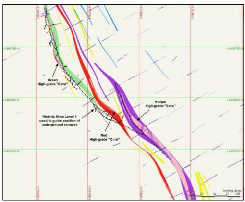
Figure 14-6: La India Deposit Plan Section 315 (Mine Level 5), showing interpreted step-across of historic mining development from hanging wall to footwall structure
