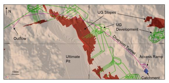
Figure 16-10: Diversion tunnel Alignment
