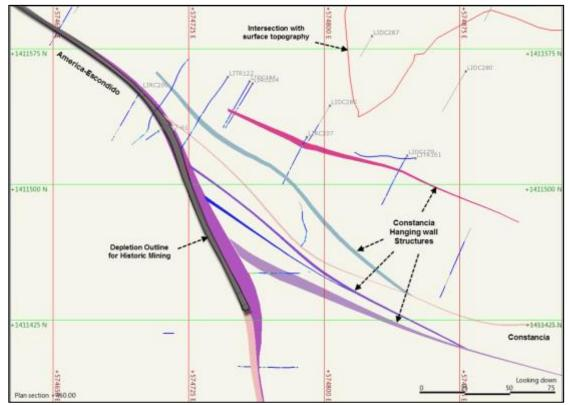
Figure 14-8: America Project Plan Section 460, showing vein strike orientation and position of the mineralisation in the Hanging wall of Constancia;
