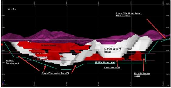
Figure 16-3: Crown and sill pillar configurations (shown with reference to La India)
