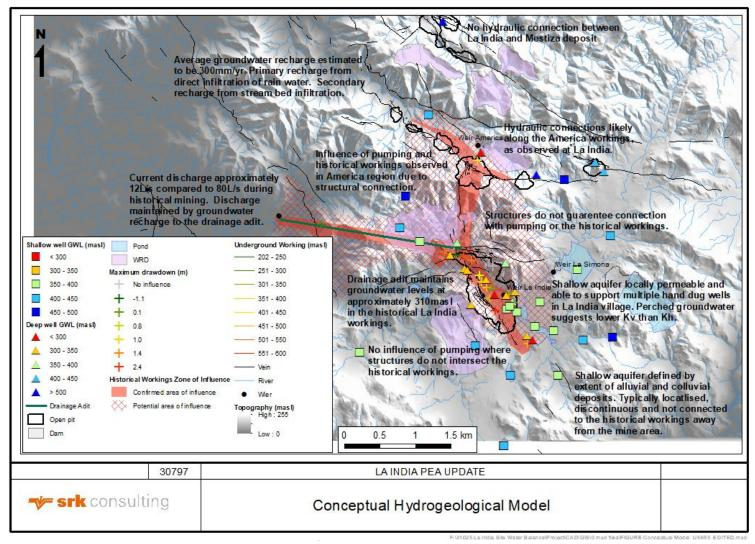
Figure 16-7: Conceptual Hydrogeological Model
