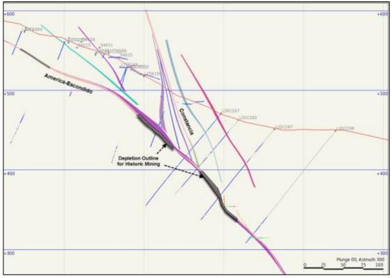
Figure 14-7: America Project Cross Section (Y=1411570), showing the junction of the America-Escondido and Constancia Veins
