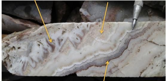
Crustiform banded quartz phases, including a chalcedonic quartz phase
